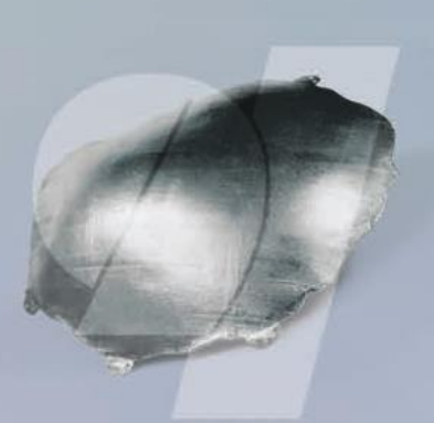
implant Ti-Al6-V4 (Grade 5)
