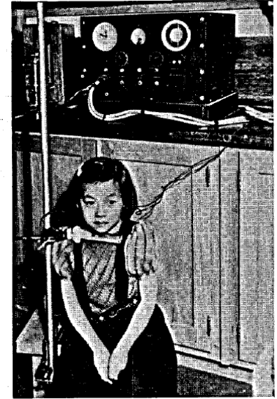
Right: The first kinetic study on the function of the human thyroid using ^{131}\text{I} and a Geiger-Muller counter.
